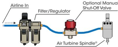
Air flow restrictions (such as air leaks) will cause underpower performance and drag your tool through the material, damaging the bearings. **Some fittings with nominal internal dimensions may have an internal diameter passage that is smaller than stated and restrict air flow and power.** It only takes one fitting with an internal diameter that is too small to reduce air flow and power of your Air Turbine Spindle®.
