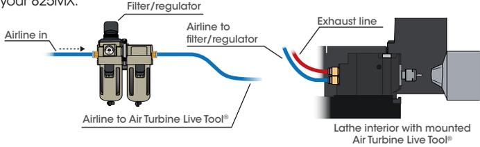
Air flow restrictions (such as air leaks and obstructions) will cause underpower performance and drag your tool through the material, damaging the bearings. **Some fittings with nominal internal dimensions may have an internal diameter passage that is smaller than stated and restrict air flow and power.** It only takes one fitting with an internal diameter that is too small to reduce air flow and power of your Air Turbine Live Tool®.
