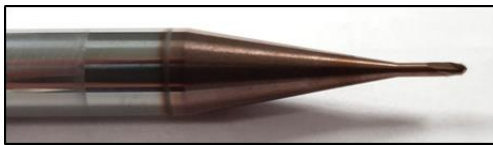
1mm ball Nose tool used during machining
