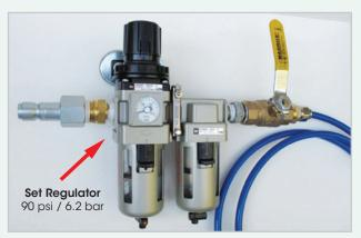
Photos of customer supplied "shut-off" valves. Ensure internal diameter meets specifications (see page 1).
