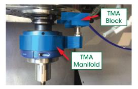
Adjust the height of the air plug using the screw mechanism to fit your machines dimensions.
