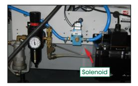
Set up a line supplying dry clean 90PSI / 6.2Bar at the rated CFM / L/S feed rate specified for your spindle in the catalog.
