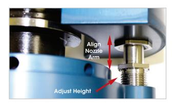
Load *Air Turbine Spindle®* carefully into CNC spindle with left hand while holding Tool Release button on CNC machine. Some trial and error may be needed, but do not let main spindle drawbar (tool release button) start unless Connector Nozzle goes up into block Inlet hole (approximately 1/4" (6mm) up into inlet hole).
