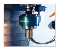
Example Model 650 Spindle loaded into CNC machine spindle. Please perform a tool change (i.e. with over-ride set to lowest speed) several times to observe the loading and unloading of the ATT spindle and ensure it engages and operates correctly.
