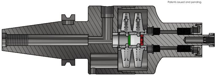
Green Position - Single Turbine Mode. Red Position - Double Turbine Mode.
